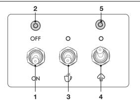
1. Power Switch : Flip down to power-on the machine.
