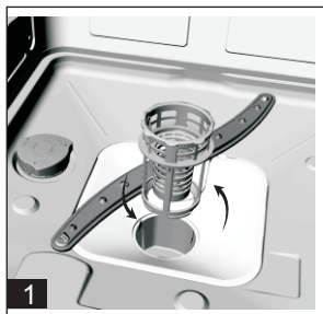
Step 1: Turn the Coarse filter anti clockwise and then lift it up. Step 2: lift the Flat filter up
